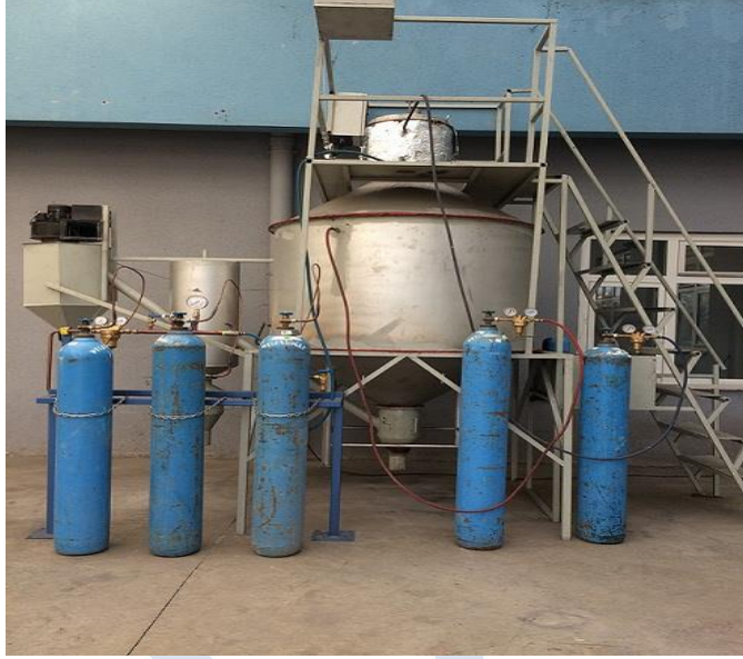
Figure 2. Karabük University Gas Atomization Unit
